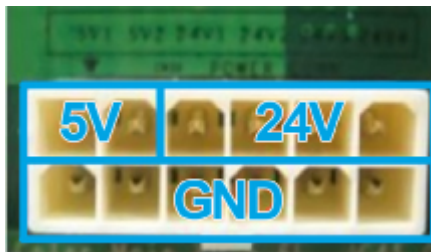
Figure 82 Main board PCA
