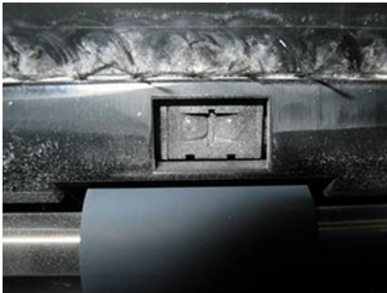
Figure 15 Example of dust contaminated sensor
