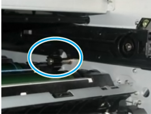
Figure 69 ITB engagement gear
