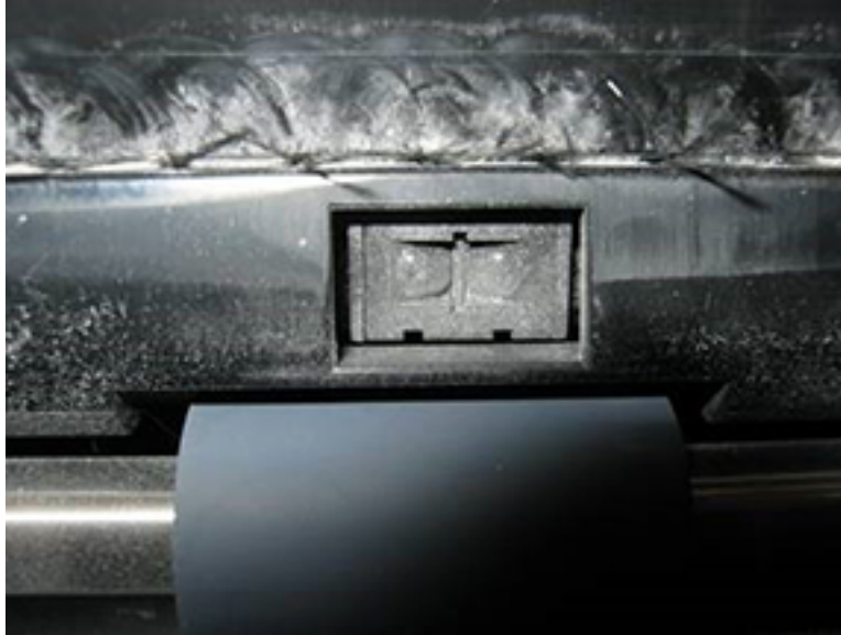
Figure 13 Example of dust contaminated sensor
