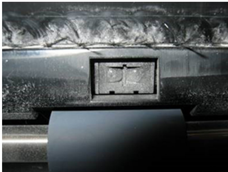
Figure 23 Example of dust contaminated sensor
